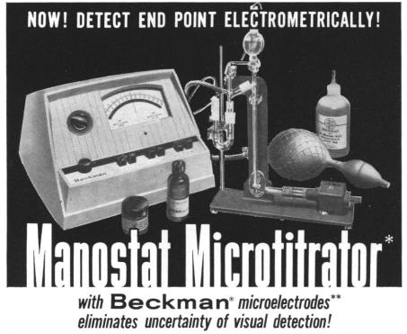
Now...titrate even a single drop-easily and accurately-with this modification of the Gilmont Ultramicroburet. Perform microtitration electrometrically, without need for visual adjust-ment of end point ment of end point.
