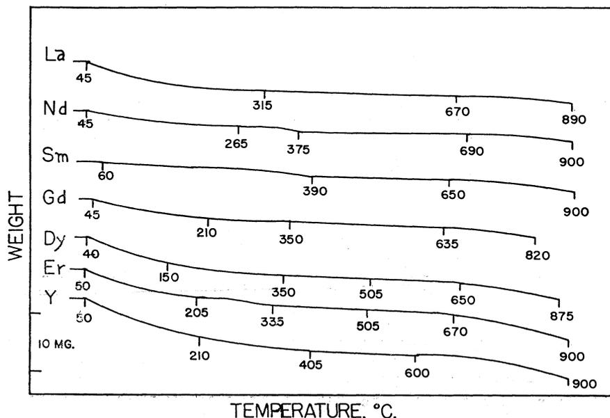
Fig. 1. Thermograms of the rare earth fluoride hydrates.
