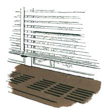
Office, classroom window sills, built with Colorlith, have unusual strength and durability . . . won't warp. Color doesn't fade. Louver slots can be readily machined.
