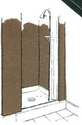
Shower stalls present a new application. Large sheets reduce number of joints. Material is strong, rigid—can't rust or deteriorate with prolonged exposure to moisture.
