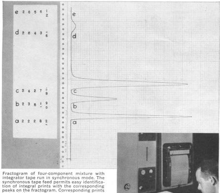
rractogram of four-component mixture with integrator tape run in synchronous mode. The synchronous tape feed permits easy identifica-tion of integral prints with the corresponding peaks on the fractogram. Corresponding prints and printing points on the fractogram are identified by letters (a, b, c, d and e).
