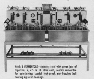
Stainless steel baths, thermostatically controlled within  $\pm \frac{1}{2}$ °C. Twin drives afford wide range of agitation and aeration rates. Machine available with automatic anti-foam addition system. Single and 3-fermentor drive assemblies also available.
