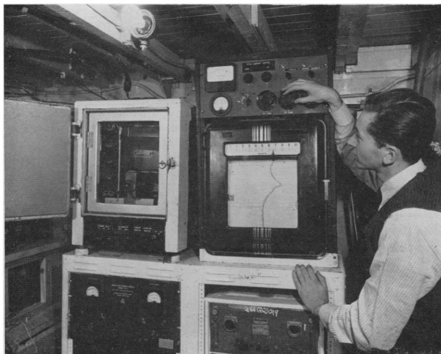
Fig. 8. The recording apparatus of a marine magnetometer—an instrument which makes continuous measurements of the earth's magnetic field—aboard the Vema , research vessel of the Lamont Geological Observatory. [National Academy of Sciences]
