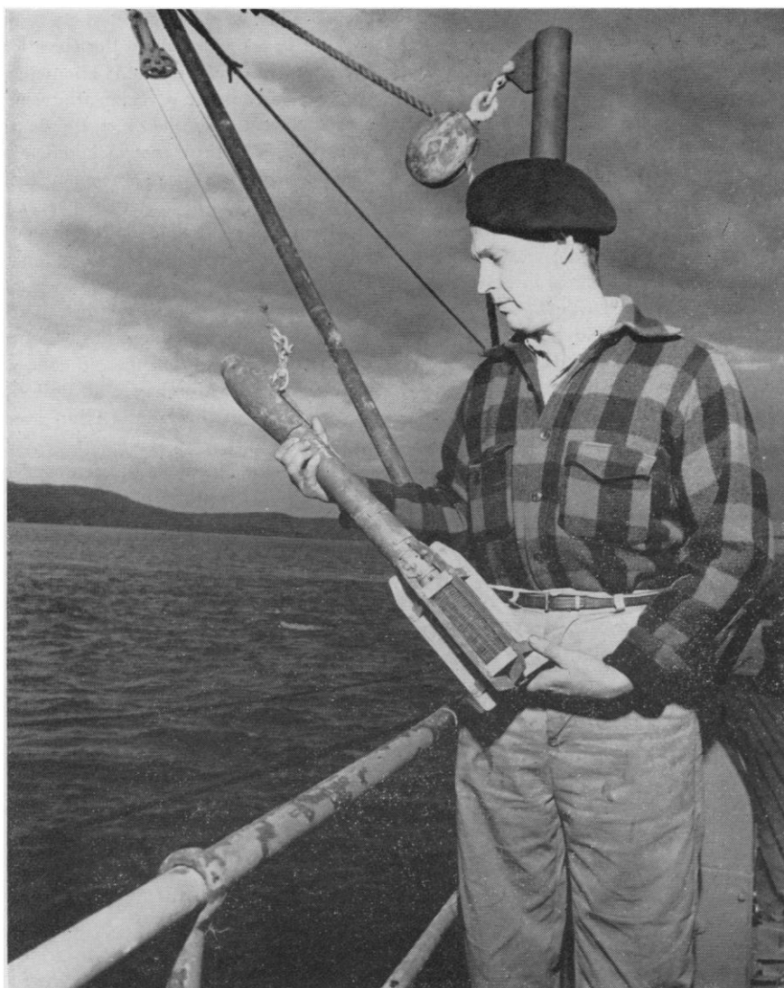
Fig. 6. An oceanographer prepares to lower a bathythermograph over the side of the research vessel Vema of the Lamont Geological Observatory. Bathythermographs record the temperature of the water at depths to 900 feet. [National Academy of Sciences]
