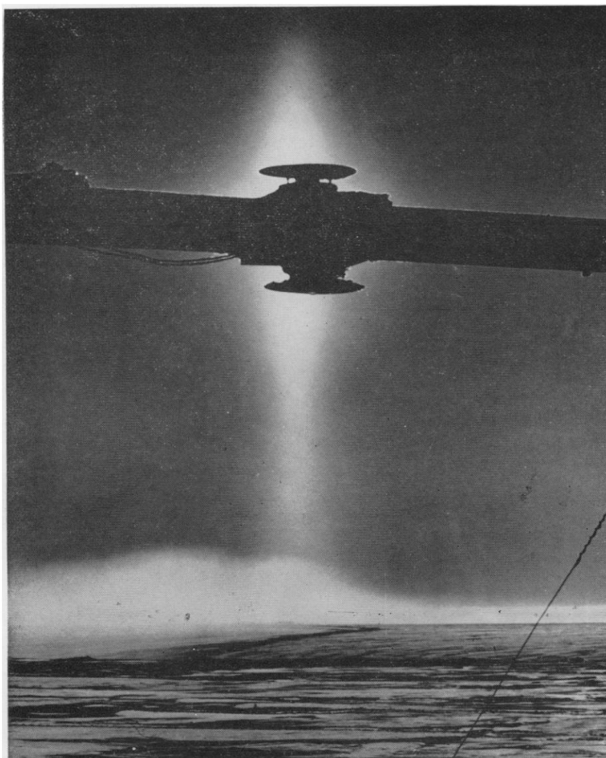
Fig. 2. Kipp and Zonen pyrhelioscopes used by Herfried Hoinkes of Austria, IGY meteorologist, at Little America station, Antarctica. The pyrhelioscopes face upward to measure incoming, and downward to measure reflected, thermal radiation. In the background is a "sun pillar"—an optical phenomenon created by the sun shining through fine ice crystals in a clear sky. [Photograph by Herfried Hoinkes]
