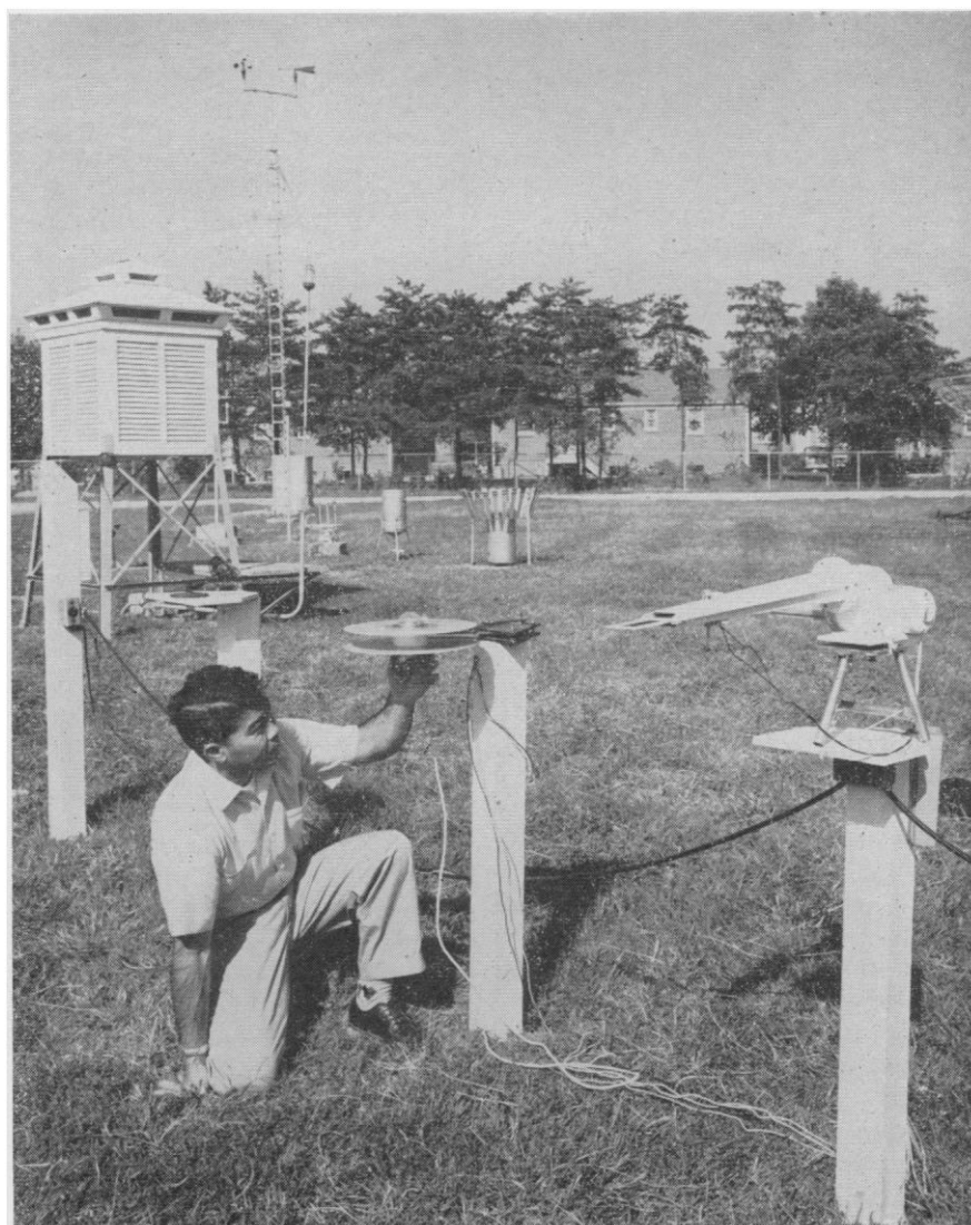
Fig. 1. A U.S. Weather Bureau observer checks the plastic shield of a Schultze radiometer. To the right is a Suomi ventilated net radiometer. The instruments in the background are a hip-roof shelter for thermometers, an anemometer and wind vane, a tipping bucket rain gage, and a weighing rain gage. [National Academy of Sciences]
