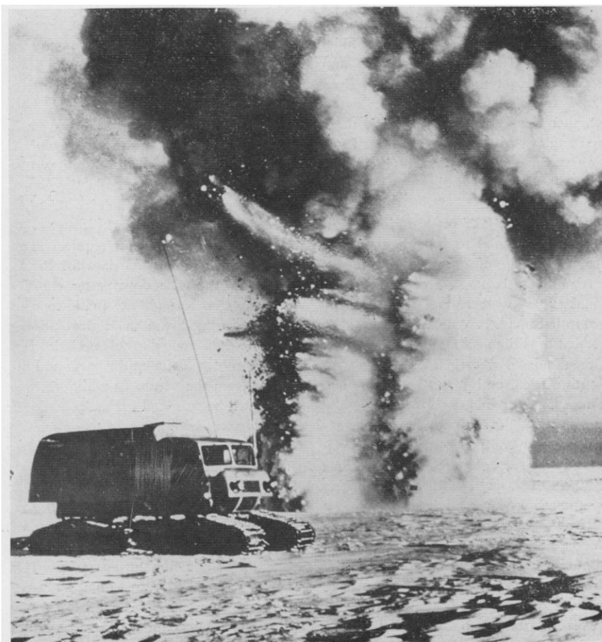
Fig. 9. Seismic explosion on the Byrd station oversnow traverse, made to determine the thickness of the ice. Shock waves from the explosion travel downward to the bedrock and echo to the surface, where they are picked up by receiving equipment. The time required for the waves to reach the bedrock and return indicates the thickness of the ice. The "sno-cat" contains the amplifiers and the recorder. [National Academy of Sciences]
