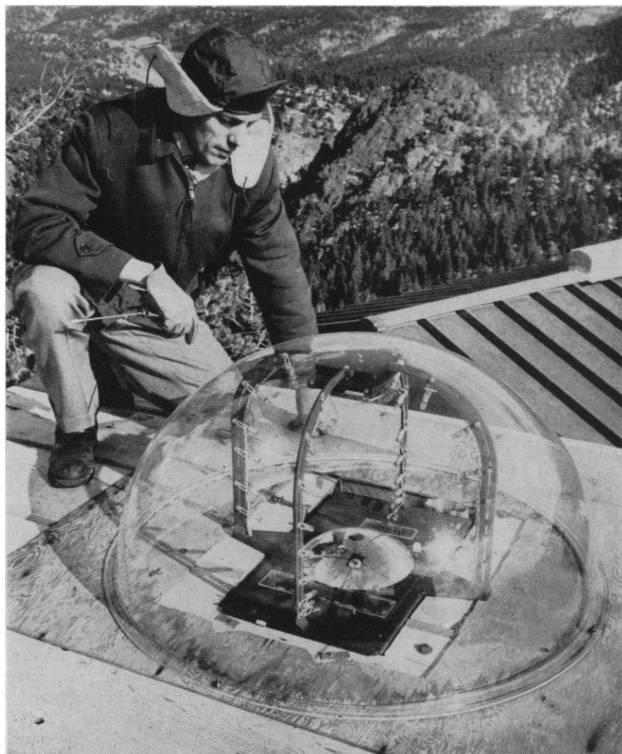
Fig. 3. Photograph taken just prior to removal of the protective plastic dome from the all-sky camera installation at Fritz Peak, Colorado, field station for the National Bureau of Standards, Boulder Laboratories. The camera, using an image from a hemispherical mirror, shown in the center, gives horizon-to-horizon sky coverage for the IGY aurora program. [National Academy of Sciences]
