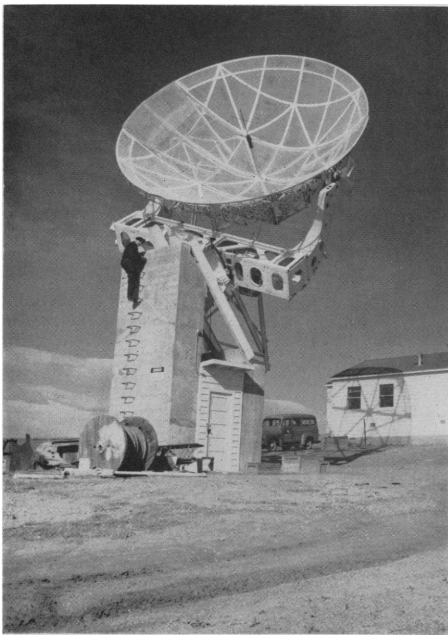
Fig. 2. One of the solar radiometers at the Gunbarrel Hill field site of the Boulder Laboratories, National Bureau of Standards. The reflector is 25 feet in diameter and is mounted so as to follow the sun throughout the day. It is in continuous operation to monitor radio noise from the sun. [National Academy of Sciences]
