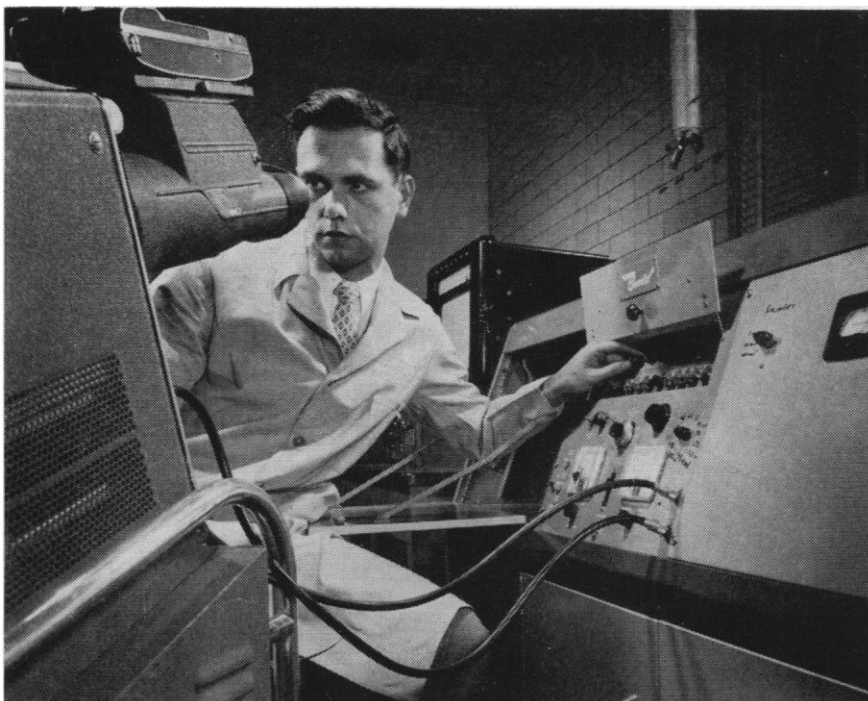
Roland Gohlke, Dow Chemical Company engineer, using Bendix Mass Spectrometer to identify compounds emerging from a gas chromatograph.
