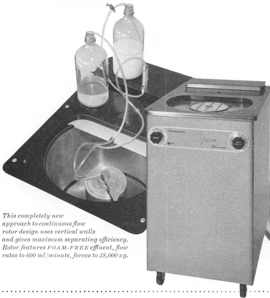
*This completely new approach to continuous flow rotor design uses vertical walls and gives maximum separating efficiency. Rotor features FOAM-FREE effluent, flow rates to 600 ml/minute, forces to 28,000 x g.*
