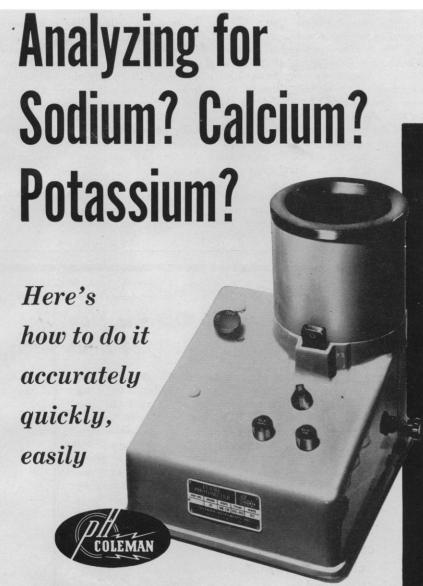
These typical industrial analyses, accomplished with a Coleman Flame Photometer, demonstrate a speed and precision impossible by classical methods:
