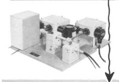
For Assay, Identification and Analysis of FLUORESCENCE—FLUORESCENCE AND TRANSMITTANCE—FLUORESCENCE AND REFLECTANCE in the Ultra Violet, Visible and Infrared Regions.
