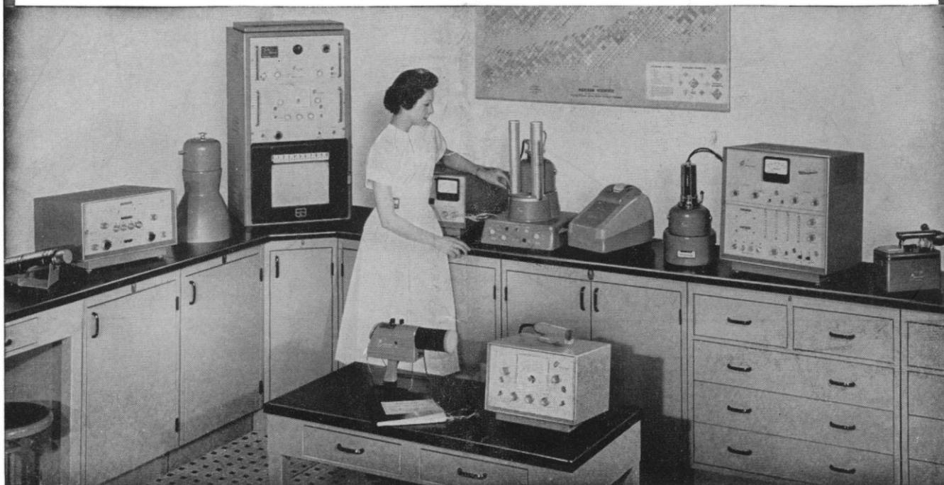
**1A** Model DS5-3P Scintillation Detector with exposed 2" x 2" sodium iodide crystal and **1B** Model 132 Analyzer Computer for precision gamma-ray measurements using pulse-height discrimination techniques.
