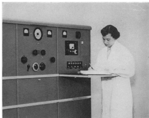
Beckman/Spinco Analytical Ultracentrifuge, Model "E." Speeds to 60,000 rpm, centrifugal forces to 260,000 G. Available with refrigeration, heating and vacuum systems; interchangeable analytical and preparative rotors; absorption, schlieren and Rayleigh fringe optical systems.
