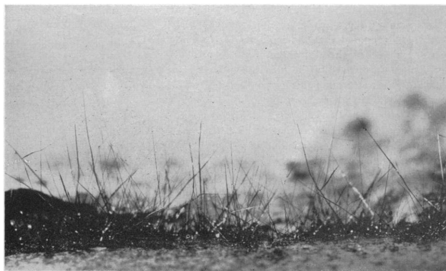
Fig. 5. Iron whiskers grown at 710^\circ\text{C} by the hydrogen reduction of ferrous bromide. (About \times 5.6 )
