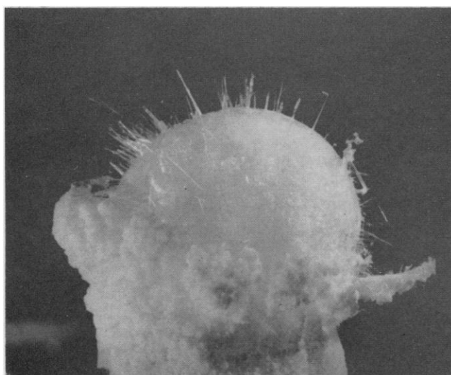
Fig. 6 (Left). Growth of NaCl whiskers on cellophane bag. (About \times 1.5 ). Fig. 7 (Right). Helical copper whisker.
