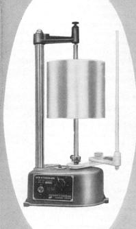
A motor driven recording drum that is very suitable for students' use and also for general experimental work.
