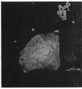
1. First, as shown in the photomicrograph\* above, the microscope analyzer was rotated until the background was brought to extinction. Readings were taken directly from the analyzer scale. Averaged settings resulted in reading of 70.4°.
