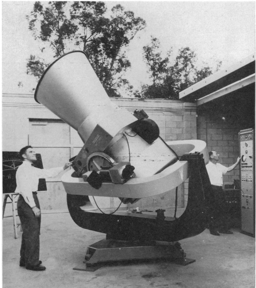
Fig. 4. A Baker-Nunn satellite tracking camera. Karl G. Henize in foreground.
