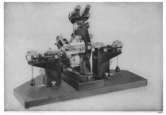
Horizontal and vertical movements of this mechanically operated instrument are independent, but can be adjusted simultaneously. Adjustable ratio of movement enables micro knives, needles, pipettes, etc., to be kept within a field of 0.1 mm. Single and double needle holders are available. Positive control of micro-instruments, without backlash, drift, or thermal expansion assured.
