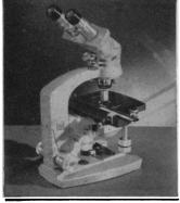
Optical path difference measurements can be made to an optimum accuracy of 1/300 wavelength. This unique ability to measure optical path thicknesses is in itself of great importance. But even more important, these measurements can be converted into a variety of quantitative information of great potential value. Water and protein content of a cell, for example, may be measured. Materials such as glass, plastics, emulsions, textiles can be examined.
