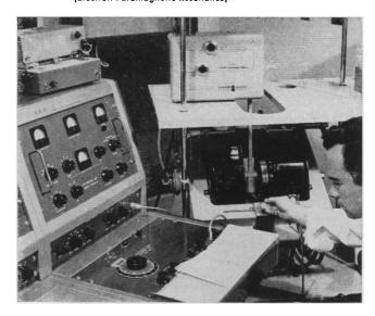
EPR spectroscopy provides the scientist with a singularly exclusive "sense." It searches the specimen and sees unpaired electrons and their environmental interactions. These may be observed in many forms: free radicals — biradicals — triplet electronic states — transition element ions — semi-conductor impurities — radiation damage sites or color centers.
