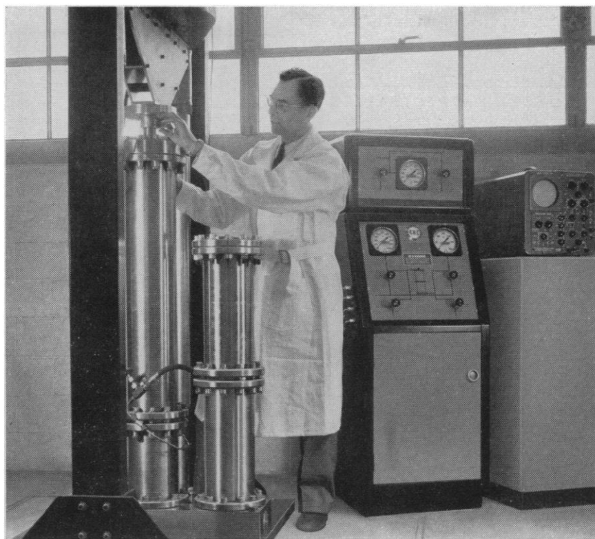
Hyge shock tester takes about 60 seconds to complete acceleration-shock test with up to 40,000 lbf. thrust. Hughes Products Memoscope® oscilloscope retains wave pattern as long as you like for careful study and comparison with master pattern.
