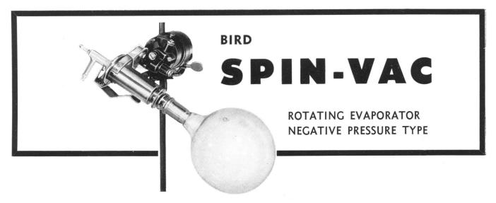
Conventional procedures for the concentration of heat sensitive compounds, biological extracts and solvents of low volatility are outmoded by the BIRD "SPIN-VAC". By employing the principle of wetting the entire inner surface of the evaporating flask, a much larger evaporating surface is obtained. This feature, plus the applying of a negative pressure, greatly speeds evaporation.
