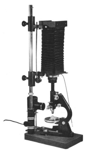
Features the standard back for 4" x 5" graphic film and plate holder. Polaroid adapter and 35 mm.
