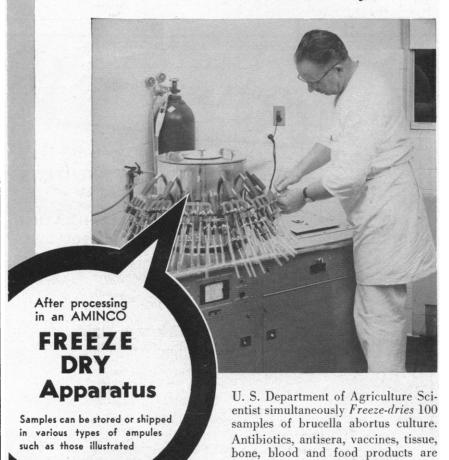
Three models available, each incorporating a stainless steel, 25-sample drying drum, and a constant reading full-range vacuum indicator:
