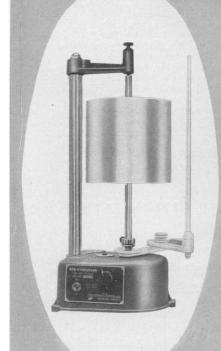
A motor driven recording drum that is very suitable for students' use and also for general experimental work.
