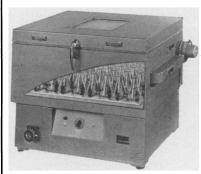
A compact, efficient self-contained, rotary action shaker and incubator featuring operation at constant temperatures with large shaking platform and vigorous agitation.
