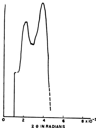
Fig. 2. Photometer trace of low-angle pattern of polyethylene (less exposure time than in the example shown in Fig. 1).
