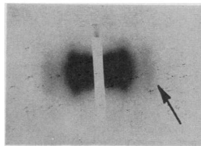
Fig. 1. Low-angle diffraction pattern of polyethylene. Copper K<sub>α</sub>, nickel-filtered radiation; specimen-to-film distance, 22.5 cm. The arrow indicates the position of the fourth order of reflection.
