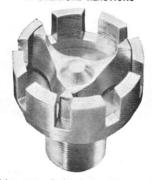
This new Swiss-designed, precisionmachined rotor-stator assembly greatly expands the usefulness of your Waring Blendor. The three-blade rotor, forcing material through the eight slots of the stator, gives you a high speed shearing action for faster mixing, homogenizing.
