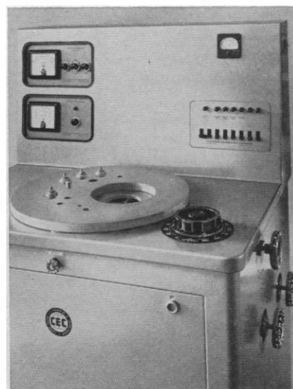
Type LC1-14A. Close-up shows control panel. Chamber: 14" by 24". Ultimate pressure: 1 \times 10^{-5} mm Hg. Diffusion pump speed: 300 liters per second at 5 \times 10^{-5} mm Hg.
