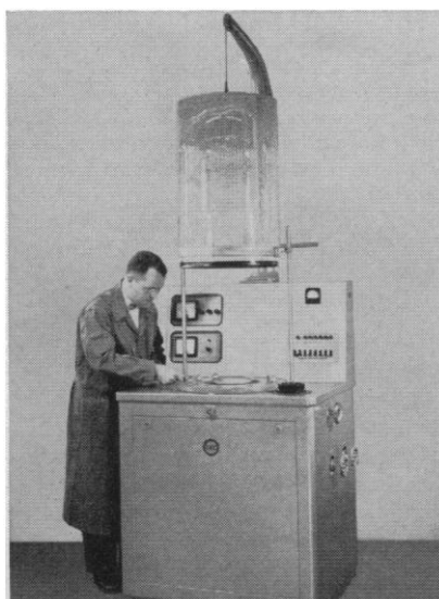
Type LC1-18A. Chamber: 18" by 30". Ultimate pressure: 2 \times 10^{-5} mm Hg. Diffusion pump speed: 475 liters per second at 2 microns.
