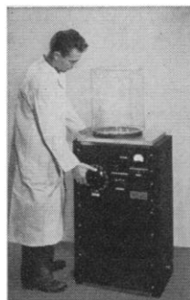
Type LC1-12A. Chamber: 12" by 18". Ultimate pressure: 1 \times 10^{-5} mm Hg. Diffusion pump speed: 200 liters per second at 5 \times 10^{-4} mm Hg.
