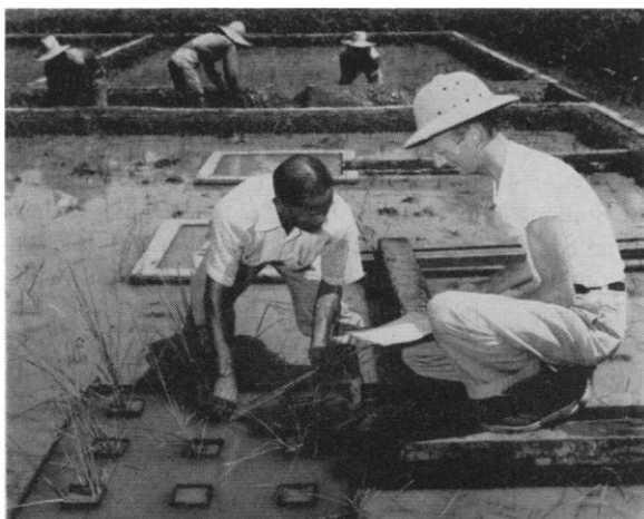
Fig. 4. Sets of tanks are used in experiments at the college's Experiment Station to find out how much water is needed by growing rice plants. The findings being recorded here by A. B. Catambay, head of the Department of Agricultural Engineering (left), and Harold E. Gray, visiting professor from Cornell, have been used to plot the most profitable and economical use of water on farms.
