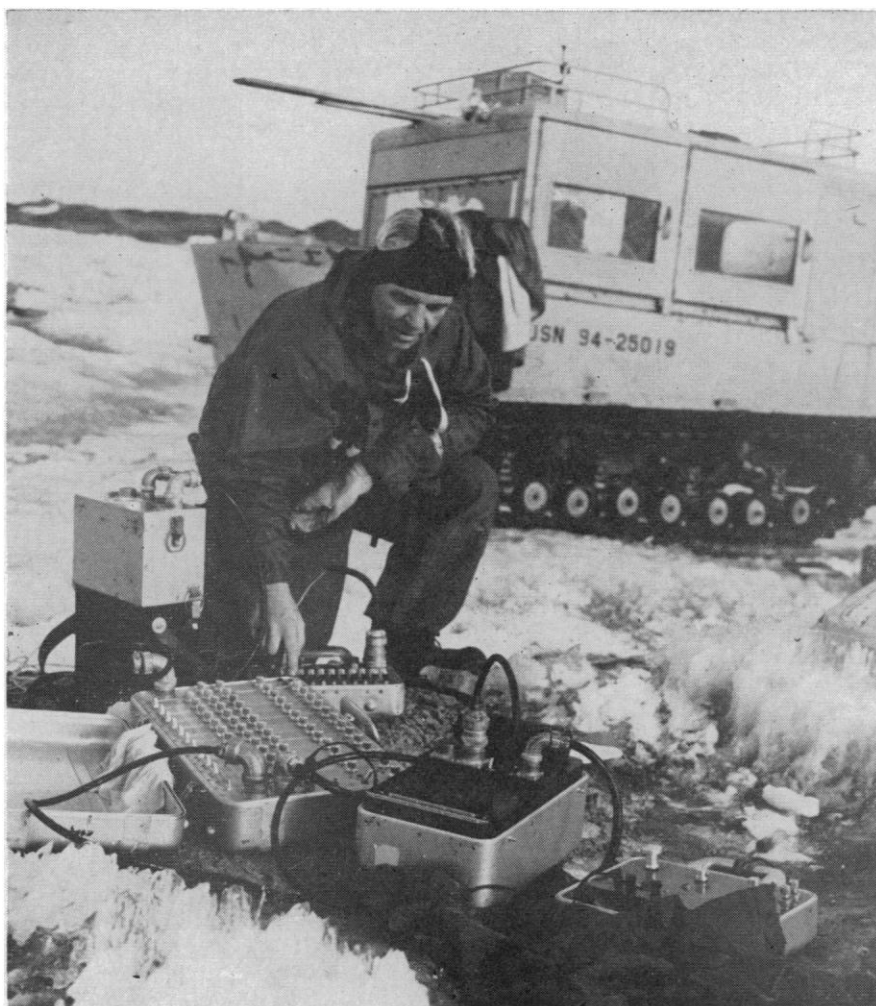
Rev. Daniel Linehan, using the 45-channel seismic recorder at Cape Roydes, McMurdo Sound, Antarctica. [D. Linehan, S. J. Weston Observatory]
