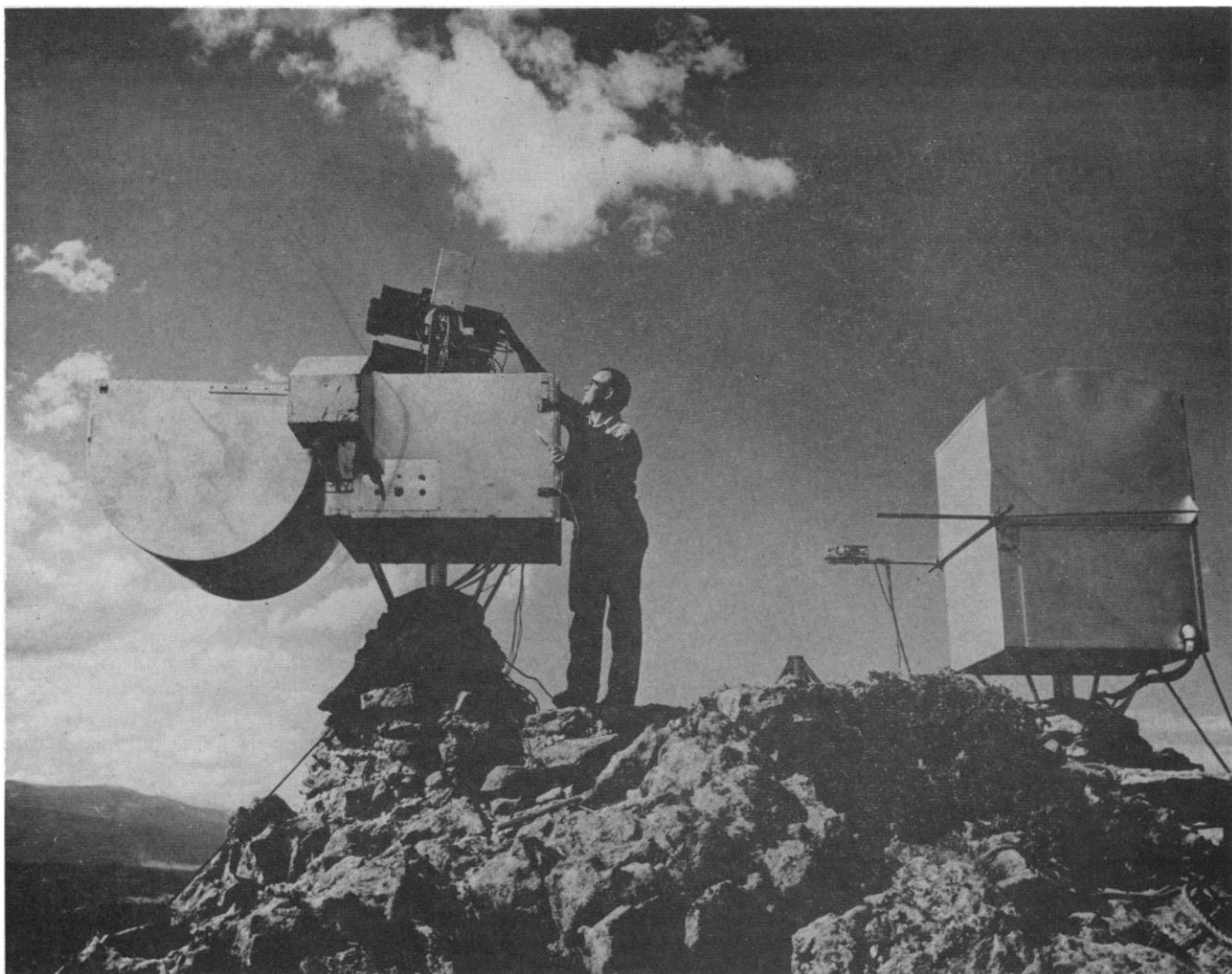
First IGY scanning photoelectric photometer, situated on top of Fritz Peak, near Boulder, Colorado. This instrument selects and measures the intensity of light too faint for the human eye to detect and records its changes, converting the light into electric signals. [National Bureau of Standards, Boulder Laboratories]
