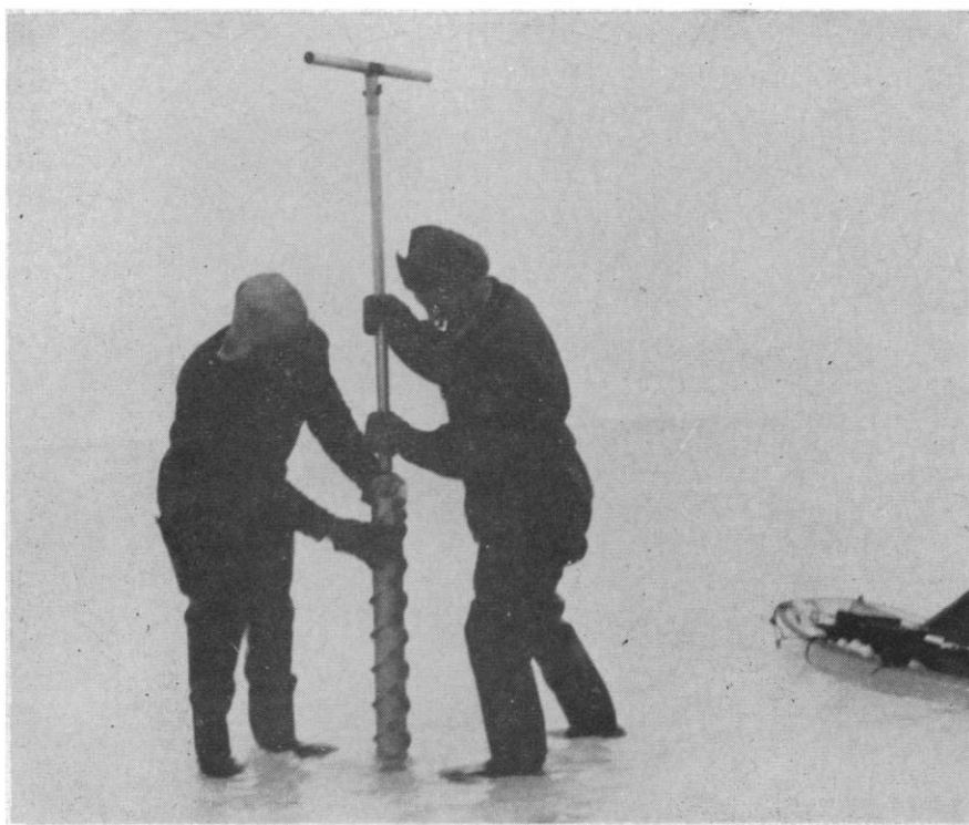
U.S. Weather Bureau scientists at IGY Drifting Station A, coring with a hand auger to drain off the "melt water"—ice which has melted on the surface. During summer months this melting ice makes construction and camp maintenance difficult. [U.S. Weather Bureau]
