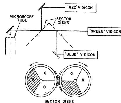
Fig. 12. Simultaneous color camera for television color-translating microscope.
