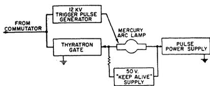
Fig. 9. Ultraviolet-source circuit.
