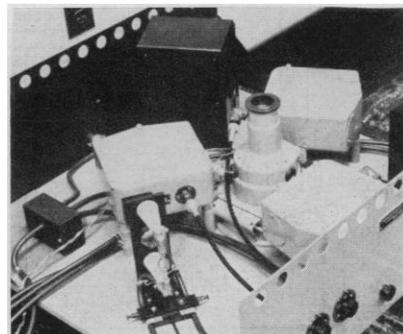
Fig. 6. Illuminating system of television color-translating microscope with three separate sources (Rockefeller Institute).
