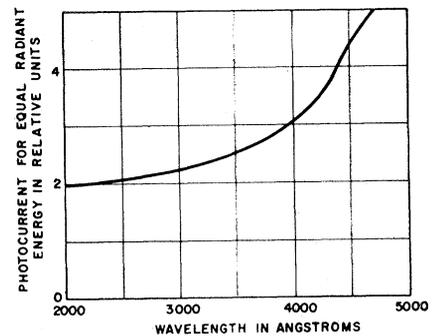
Fig. 2. Ultraviolet response of experimental ultraviolet-sensitive Vidicon.
