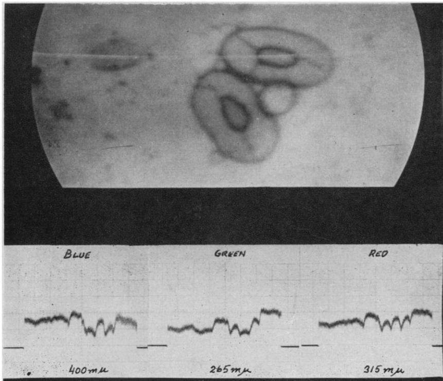
Fig. 11. Red cell of frog blood and oscillograms representing transmission at three ultraviolet wavelengths along selected scanning line.
