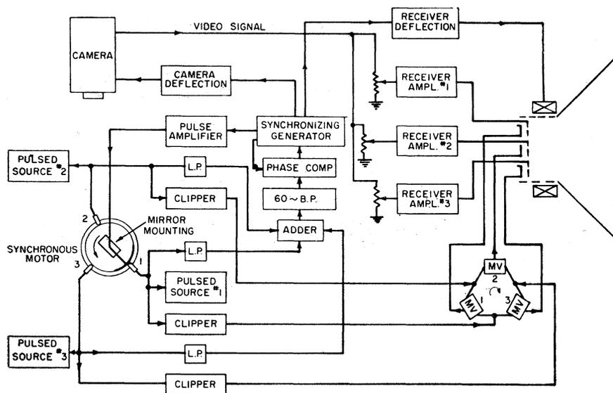
Fig. 8. Block diagram of television color-translating microscope at Rockefeller Institute for Medical Research.
