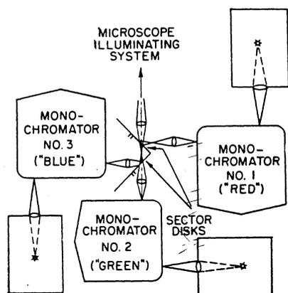
Fig. 13. Sector-disk illuminator for television color-translating microscope.
