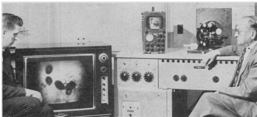
Fig. 10. Complete television color-translating microscope (Rockefeller Institute).
