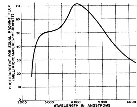
Fig. 3. Ultraviolet response of experimental ultraviolet-sensitive image orthicon.
