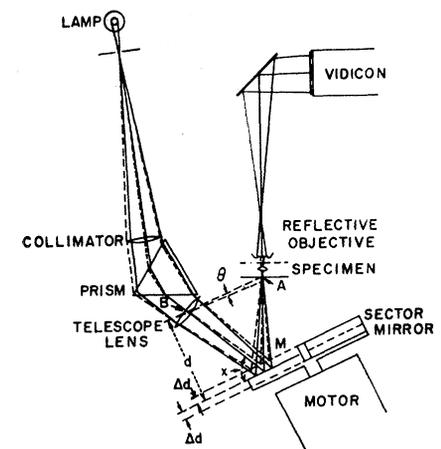
Fig. 4. Optical system of single-source television color-translating microscope.
