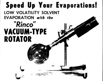
You can step up your rate of evaporations four or five times without bumping with a Rinco Rotating Vacuum-Type Evaporator. It is especially successful with solvents such as dimethylformamide and water. Thirty mloof water at 22°C. will evaporate in approximately 20 minutes.
