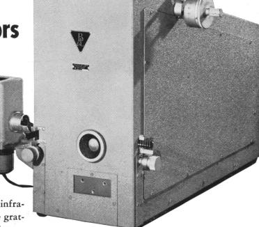
Pure, intense light . . . ultra-violet, visible, or infrared—just turn the micrometer drum to set the grating to the desired wavelength. Wide choice of gratings for full range coverage (2000A-14,000A), or for more intensive U-V or infra-red study. Nine monochromator models, with linear dispersion from 66A/mm to 16.5A/mm, first order.
