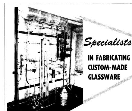
High vacuum Apparatus for the Determination of Surface Area by the Brumauer-Emmett-Teller Method operating in the plant of C. K. Williams & Company. Easton, Pennsylvania, The apparatus, for measuring gas adsorption isotherms, is made of "Pyrex" brand glass. It was designed in cooperation with the Surface Chemistry Laboratory of Lehigh University.
