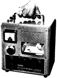
The Cahn Electrobalance is easy to operate, fast, rugged and portable, yet has accuracy equal to many delicate microbalances. Balancing time takes but a second or two. Complete weighings average less than a minute. Readings are taken directly in micrograms.
