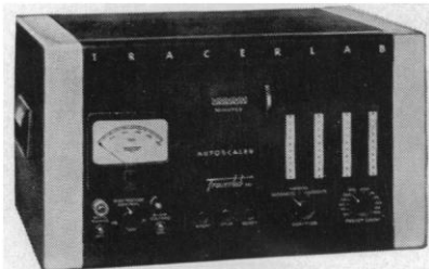
SC - 51 AUTOSCALER ... first all-electronic laboratory scaler for automatic counting, either binary or decade.
