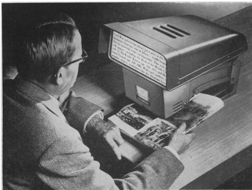
Fig. 1. Use of the projection magnifier, reading device for the partially sighted.
