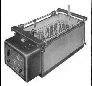
Standard interchangeable trays are provided in several styles to accommodate different sizes of flasks in the reciprocating rack. Racks are easily removable and are adjustable.
