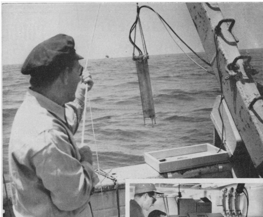
(above) Nuclear-Chicago scintillation detector is lowered into water for tracing the radioactive sewage effluent at varied depths over a 25 square mile area. (right) Gamma-ray spectrometer system, ratemeter and recorder on laboratory ship measure and chart traces of radioactive scandium during 36-hour period of experiment.
