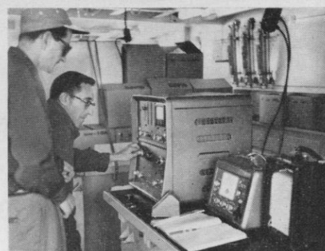
(above) Nuclear-Chicago scintillation detector is lowered into water for tracing the radioactive sewage effluent at varied depths over a 25 square mile area. (right) Gamma-ray spectrometer system, ratemeter and recorder on laboratory ship measure and chart traces of radioactive scandium during 36-hour period of experiment.
