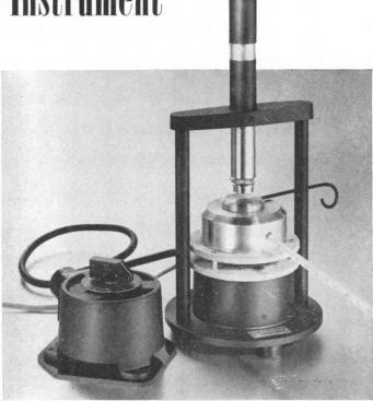
This new precision instrument was developed with the help of Dr. Leonard R. Axelrod of the University of Rochester School of Medicine and Dentistry, to determine with precise accuracy the melting points of single crystals. It consists of a 25 power microscope with polaroid inserts, built-in light source, aluminum block with 200 watt heating element and a thermometer seated within hot stage in close proximity to sample to insure positive accuracy of readings.
