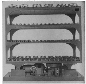
A large capacity shaking apparatus of unique design which assures positive linear and uniform motion on all tiers. It has a variable speed range of 38-125 strokes per min. and an adjustable stroke of  $0^{\prime\prime}-4^{\prime\prime}$ . An automatic pressure feed lubrication system simplifies maintenance. Available with removable trays equipped with various types of clamps or other holding devices.
