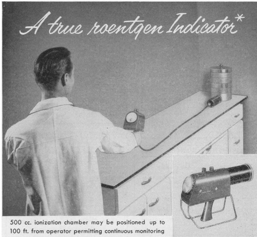
500 cc. ionization chamber may be positioned up to 100 ft. from operator permitting continuous monitoring of high radiation intensity without hazard to personnel.
