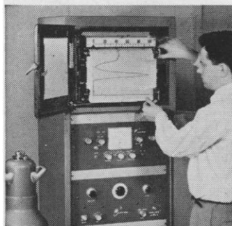
Automatic scanning and recording of spectrum energies is accomplished by Analyzer, rate-meter, recorder and scintillation counter. Gamma energy spectrum of Cesium-137 is shown on recorder chart.
