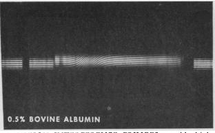
RAYLEIGH INTERFERENCE FRINGES provide highsensitivity measurement of solute concentration at any level in analytical cell. Used for determining molecular weights both high and low—by the equilibrium method, as well as for measuring sedimentation velocity by the centrifugal trans port of material past a given level in the cell.
