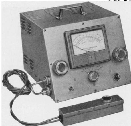
For the exact measurement of light values as low as 1/10,000 microlumen . . . for absorption and flame photometry, colorimetry through microscopes, scintillation measurements, fluorescence trace analysis, etc.
