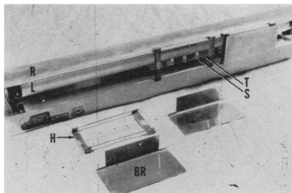
Fig. 1. Ultraviolet sun lamp assembly for the photopolymerization of monomeric methacrylates. *BR*, backing reflector; *H*, specimen holder; *L*, fluorescent sun lamp; *R*, reflector; *S*, specimen capsule; *T*, cellophane tape.
