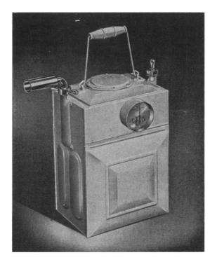
For respiratory tests and evaluation of patients who face operations within the chest . . . The force required to operate this meter, either pressure or vacuum, is only a fraction of an ounce per square inch. Consequently it is ideally suited for the determination of lung capacity . . . Index reads from .01 to 1,000 liters. Large dial pointer makes one revolution per liter.
