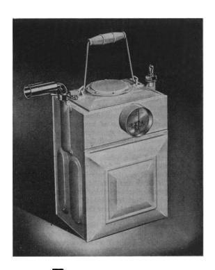
For respiratory tests and evaluation of patients who face operations within the chest . . . The force required to operate this meter, either pressure or vacuum, is only a fraction of an ounce per square inch. Consequently it is ideally suited for the determination of lung capacity . . . Index reads from .01 to 1,000 liters. Large dial pointer makes one revolution per liter.
