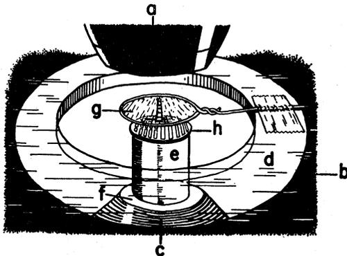
Fig. 3. Equipment used to transfer the serial sections to a Sjöstrand grid: *a*, microscope objective lens; *b*, microscope stage; *c*, condenser; *d*, large plastic disk; *e*,  $\frac{1}{8}$ -in. plastic rod; *f*, plastic disk to support rod; *g*, loop with serial sections; *h*, Sjöstrand grid.
