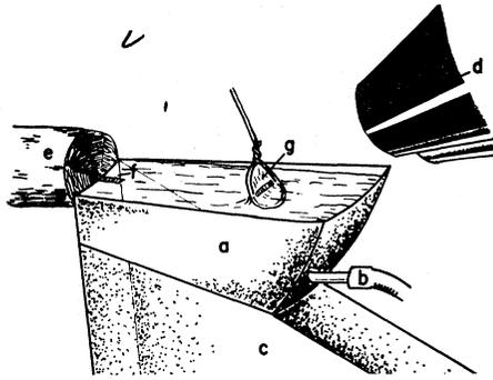
Fig. 2. Equipment used to collect serial sections: *a*, collecting trough; *b*, plastic tube connecting the trough with the hypodermic syringe; *c*, glass knife; *d*, dissecting microscope; *e*, methacrylate block; *f*, ribbon of serial sections; *g*, Formvar-coated loop
