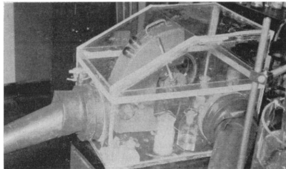
Fig. 1. An apparatus for determining refractive indices in an oxygen-free atmosphere.
