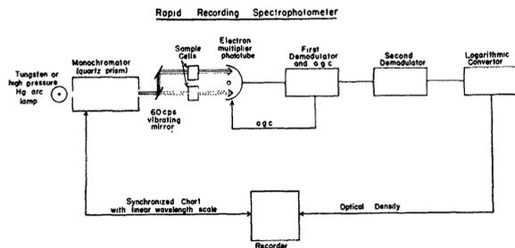
Fig. 4. Split-beam recording spectrophotometer constructed to measure difference spectra. The vibrating mirror is mounted on a Brown "Converter" and its switch contacts select wave forms of the photomultiplier output corresponding to the two-beam positions.
