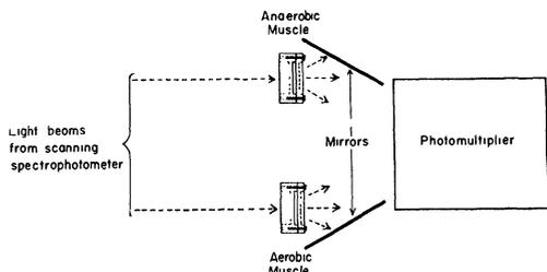
Fig. 3. Optical arrangement suitable for measuring the reduced-oxidized spectrum for the respiratory pigments of a pair of frog sartorius muscles.
