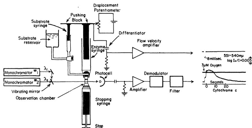
Fig. 16. The regenerative flow method for the measurement of very rapid chemical reactions in suspensions of intact cells in the particular experimental result shown at the right, anaerobic yeast cells are mixed with  $3 \mu\text{M}$  oxygen, and the oxidation of the intracellular ferrocytochrome *c* is recorded by the double-beam spectrophotometer.
