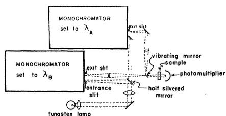
Fig. 1. Double-beam spectrophotometer using quartz or grating monochromators. The sample volume is 0.8 to 10 ml. The vibrating mirror is mounted in a Brown Instrument Co. "Converter" and oscillates at 60 cy/sec.
