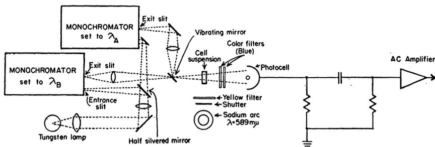
Fig. 13. A modification of the apparatus of Fig. 1 for spectroscopic measurements of the kinetics of photochemical reactions. The capacitance coupling in the amplifier, together with the blue filters, renders the measurement circuit insensitive to the illumination of the cell suspension with yellow light.
