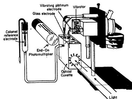
Fig. 5. Arrangement permitting simultaneous measurement of respiration with the platinum electrode, fermentation by means of the change of pH in a lightly buffered medium as recorded by the glass electrode, and changes in the steady-state levels of the respiratory enzymes by the double-beam spectrophotometer.
