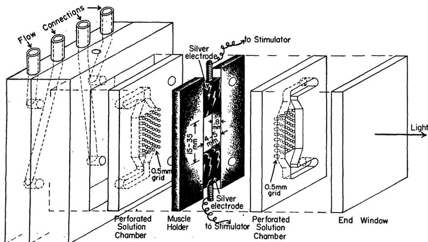
Fig. 18. Flow chamber for spectroscopic observations of changes in the steady-state level of reduced pyridine nucleotide enzyme systems in aerobic frog sartorius muscle. The flow chamber is made of Lucite (free of ultraviolet-absorbing dyes).
